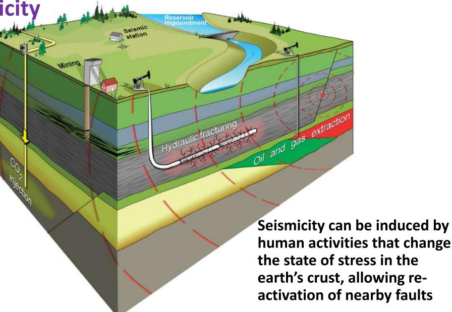
Figure 2. Potential sources of induced seismicity (reservoir impoundment, mining, oil and gas extraction, hydraulic fracturing, fluid or gas disposal or injection for enhanced oil recovery).
