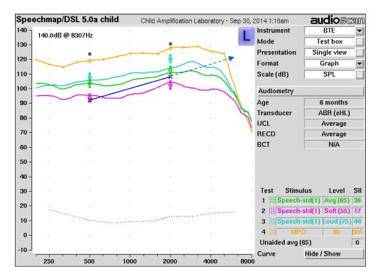
**Figure 9.** Text box measurements of soft (pink), average (green) and loud (blue) and for the MPO (yellow) measured at a presentation level of 65 dB SPL.
