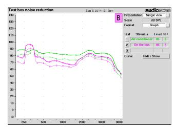
When the noise management strategy is enabled, an average of 6 dB noise reduction is noted when 'Air conditioner' and 'On the bus' signals are delivered to the hearing aid. Other noise reduction stimuli available in this system include 'Vacuum' and 'Multitalker Babble'.
