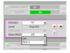
Specific stimuli and procedures integrating the MAOF concept are recommended in this protocol (Glista, et al., 2016; Scollie et al., 2016). A display of peak and valley measurements for the LTASS is needed when identifying the MAOF range.
