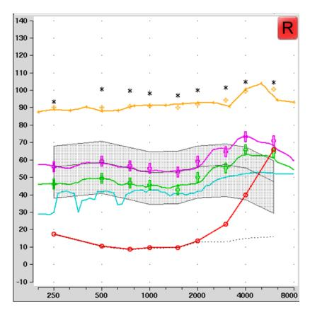
**Figure 3.** An example of a low-gain hearing aid fitting. The x-axis is frequency (Hz) and the y-axis is sound pressure level (SPL) at the eardrum. The blue line is the hearing aid's noise floor which may be heard by the listener. Note that soft aided speech (green line) is not much better than the noise floor. The SII values for average aided speech (pink line) is 94% and the SII values for soft aided speech are 89%.
