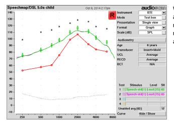
When a loud speech input is delivered to the hearing aid with noise management, the hearing aid maintains a good fit to DSL targets. Therefore, the noise management strategy does not impact the audibility of speech in quiet:
