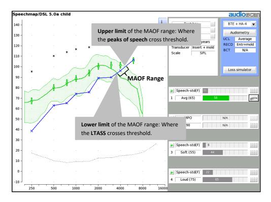
**Figure 2.** An Audioscan® Verifit2 test box screen measurement of the LTASS (with peak and valley measurements displayed) in reference to the hearing threshold line for an average level presentation level. The MAOF range extends from the point where the LTASS crosses threshold to the point where the peaks of speech cross threshold.
