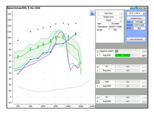
**Figure 7.** Text box measurements of the LTASS (green) and /s/ (pink) and /ʃ/ (blue) at a stronger setting, for a presentation level of 65 dB SPL.
