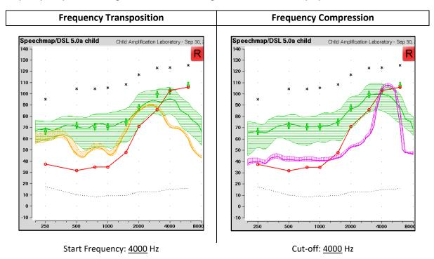
In this example, frequency transposition has lowered the peak of /s/ to approximately 3000 Hz whereas frequency compression is lowering to around 5000 Hz despite both using a setting of 4000 Hz. Due to the processing applied to the signal, frequency transposition appears to provide more lowering than frequency compression at the same setting.
