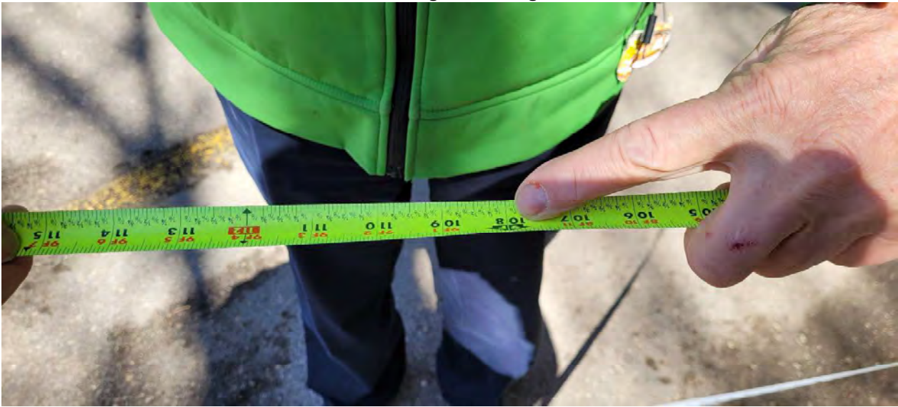
Photo 2: Existing Clearance – 9’ (2.7 m)
