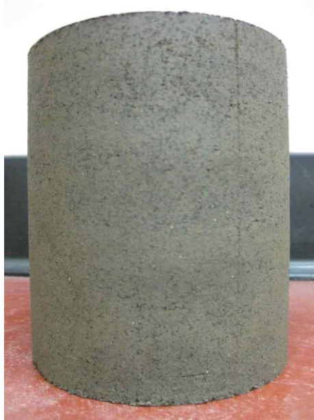
FIG. 2-A compacted specimen of mine tailings and small tire crumbs mixtures with the mixing ratio of tire crumbs of 0.2 and the water content of 15% (i.e., TC0.2-SP-S-W15).
