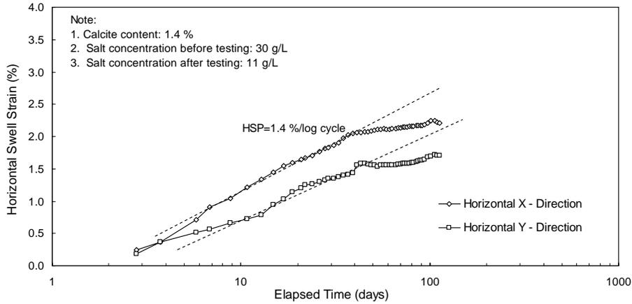
Figure 4. Results of free swell tests (Shale, Kentucky)
