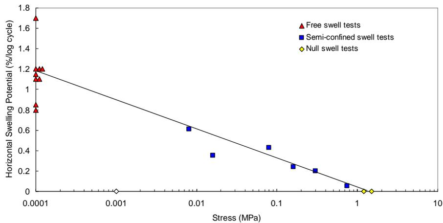
Figure 5. Suppression pressures from results of semi-confined and null swell tests (Shale, Kentucky)
