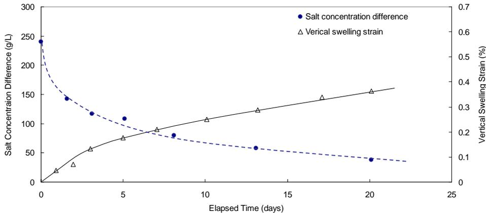
Figure 3. Change in salt concentration and vertical swelling strain with time (Queenston shale, Ontario; after Lee and Lo, 1993 [4])
