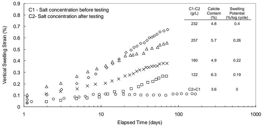
Figure 2. Results of free swell tests under different salt concentration between the pore fluid and the ambient fluid (Queenston shale, Ontario; adopted from Lee and Lo, 1993 [4])
