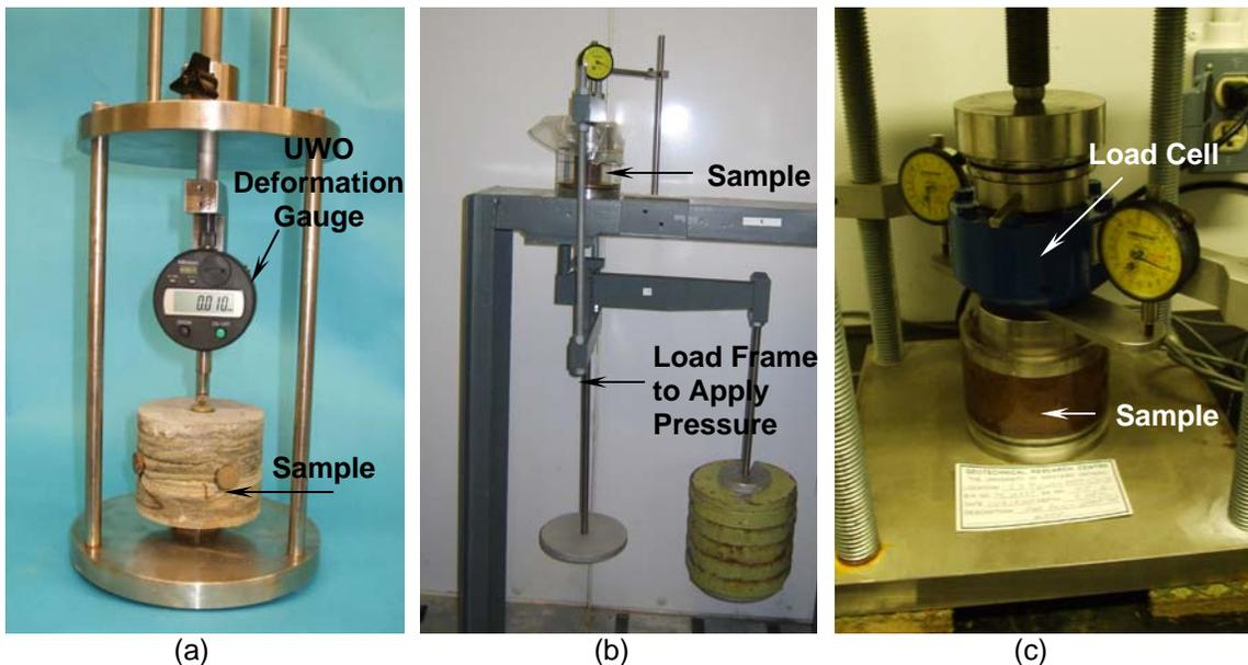
Figure 1. Swell tests set-ups: (a) free swell test, (b) semi-confined swell test and (c) null swell test
