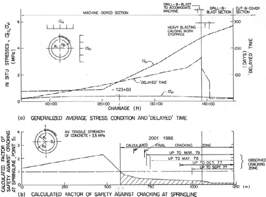
Figure 8. History of cracking along tunnel (Heart Lake Tunnel, Ontario; adopted from Lo and Yuen, 1981 [10])
