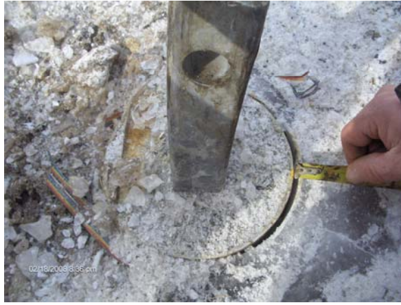
Fig.13. FRP-G-HSP with external grout separation between the FRP tube & external grout during lateral testing
