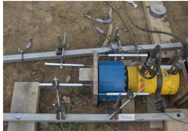
Fig.12.b. Lateral loading setup zoom-in
