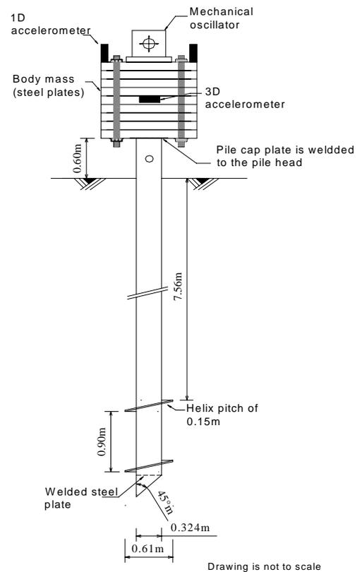
Figure 3. Pile-mass system
