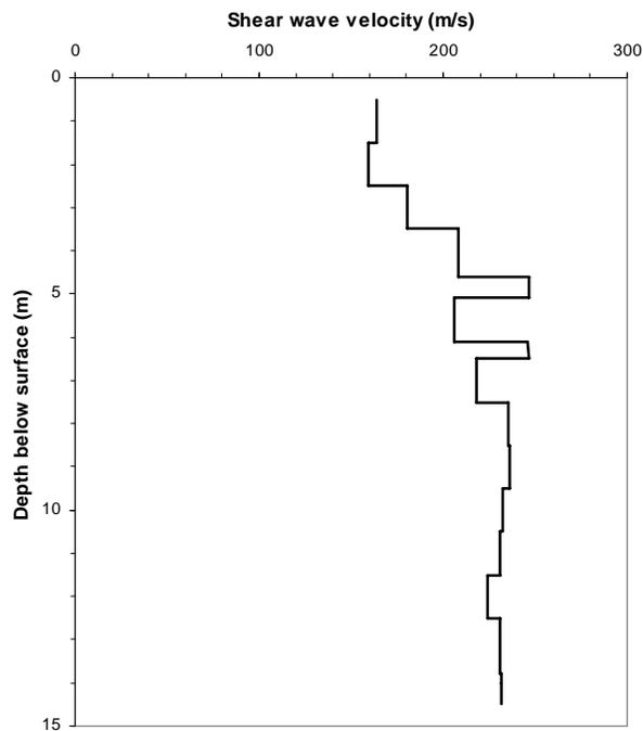
Figure 2. Shear wave velocities distribution
