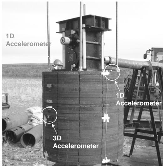
Figure 5. Location of accelerometers
