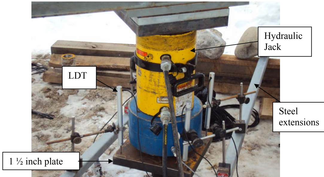
Figure 8. Instrumentation at the pile head
