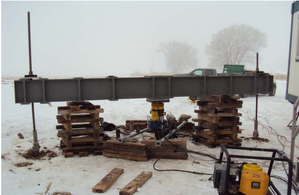
Figure 6. Compression Load test setup
