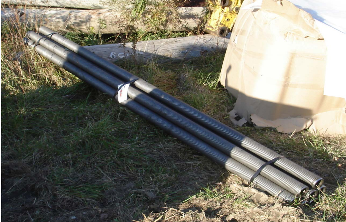
Figure 4. B7X1-76 Geo-drilled Hollow Core Anchors
