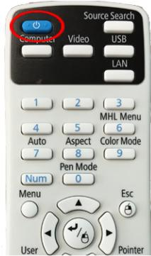
2a. Once powered on press the "LAN" button on the projector remote.
