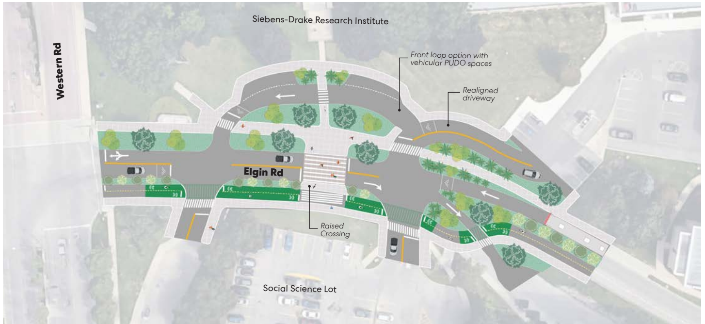
Figure 75. Conceptual Sketch of New PUDO/Turnaround at the Siebens-Drake Research Institute – Option 2 – West Side Pull Through
